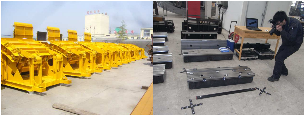
Moulds with an exterior diameter of 6000 mm for Guangzhou Subway / Photometric control of moulds by GOM
